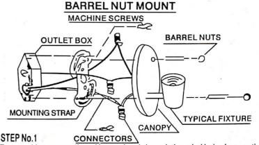
Turn machine screws (found in envelope) through threaded holes in mounting strap as shown.
