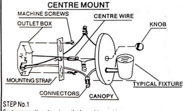
Fasten mounting strap to outlet box with machine screws (found in outlet box).
